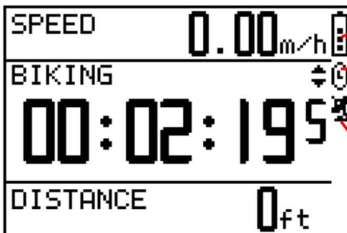
The battery icon indicates the remaining battery power.
