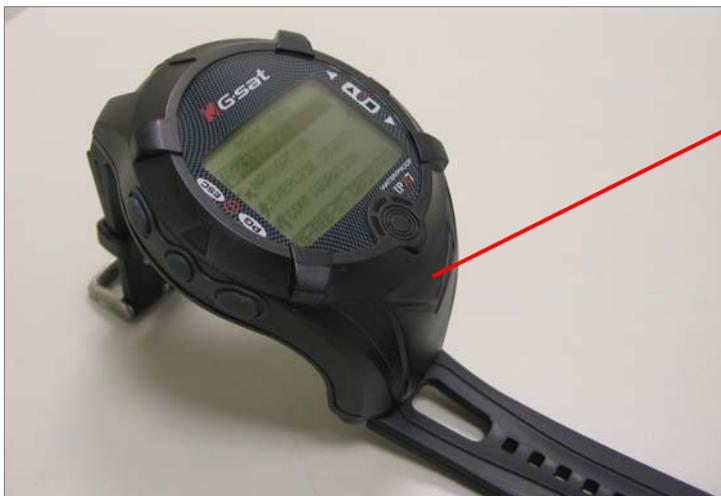
The GPS antenna is located in the lower part of the device. Let it face to the sky for a better reception.
