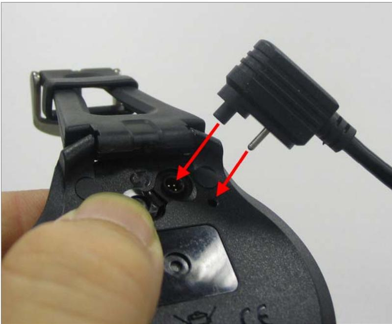
Connect the USB cable as shown on left figure.
